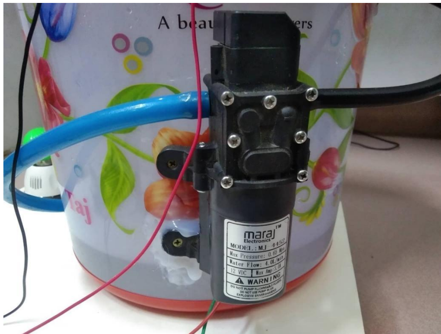
Figure 3.13: High Speed Pump
