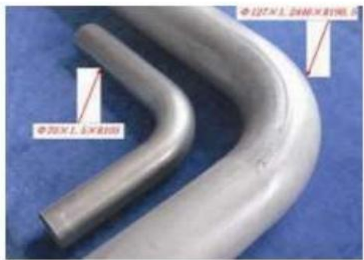
Figure 2.10: Experimental bent tubes with large diameter (Hea, 2012)
