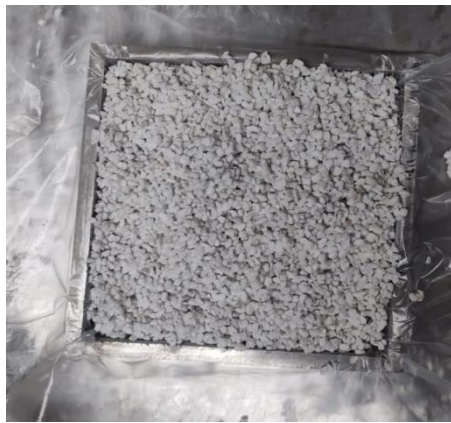
(b) Pouring perlite mixture inside the mold
