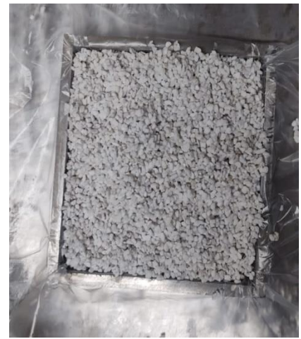
(c) Placing the core up on the lower skin
