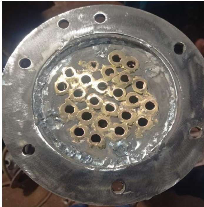
Fig: 5 (Copper tubes are fixed with tube sheet)
