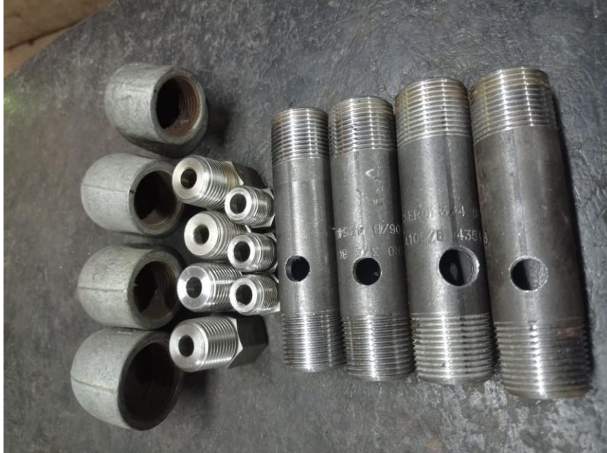
Fig:14 (Temperature Indicator-TI fittings)
