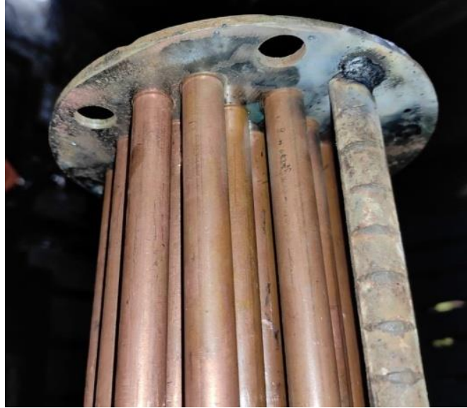
Fig: 4 (Copper tube and tie rod)
