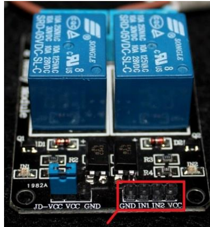
Figure 3.16: Main Voltage Connection
