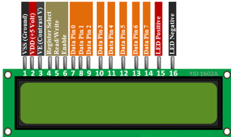
Figure 3.10 16x2 LCD connection
