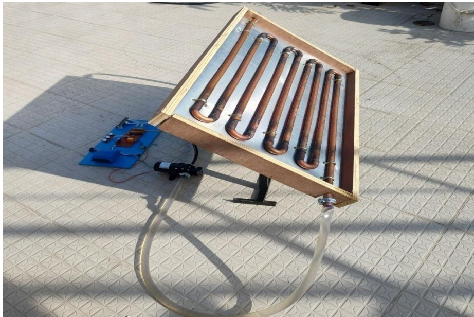
Figure 1 Solar Heater system
