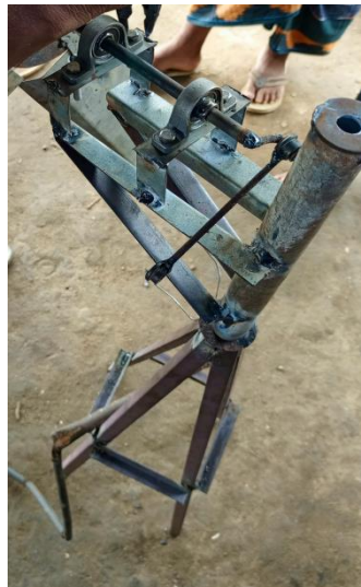
Figure 4.18 Connect The Hub With Shaft And Crank Shaft
