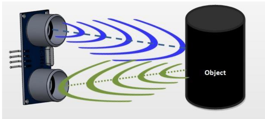
Figure 3.22: Ultrasonic Sensor Working Procedure
