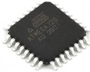
Figure 3.5: Micro controller IC AT Mega 328p
