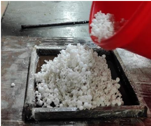
Figure 13 Watted EPS and EP Pouring
