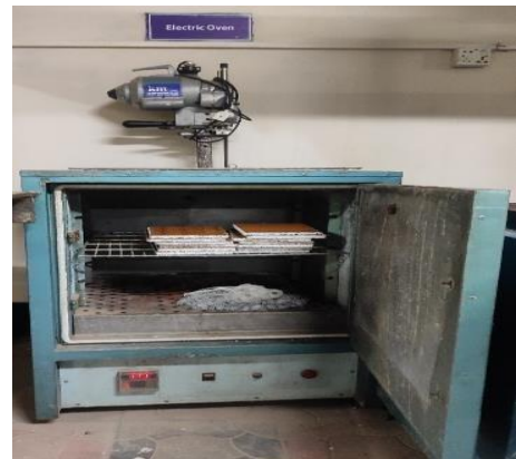
Figure 24 Drying in woven for evaporation of Acetone
