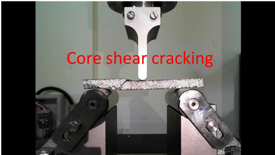
Figure 31 core share and cracking sample EPS-0,EP-100
