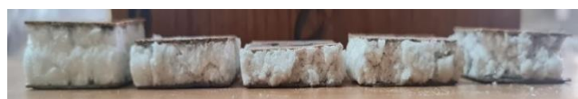
Figure 39 shows images of specimens that failed the compression test, ranging from EPS100-EP0 (on the left) to EPS0-EP100 (on the right)
