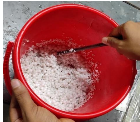
Figure 11 Wetting Dry EP & EPS with (ERS)
