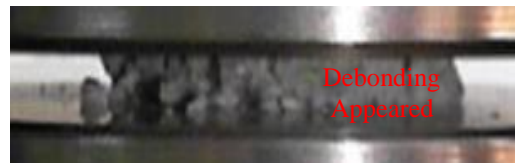
Figure 38 shows images of specimens that failed the compression test EPS-0,EP-100
