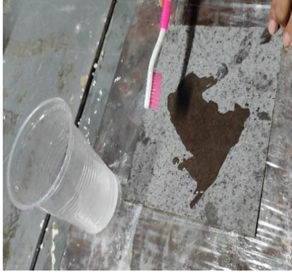
Figure 16 Wetting Dry EP & EPS with (ERS)
