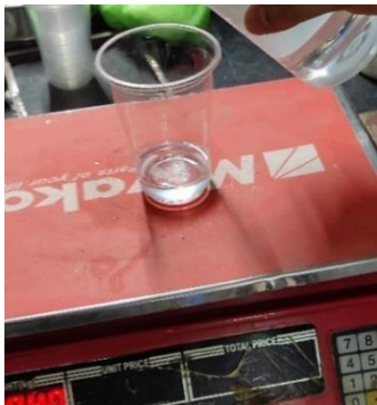
Figure 10 Epoxy-Resin Solution (ERS) preparation.
