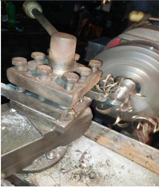
Continuous chips during turning operation
