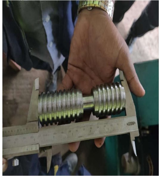
Prepare lathe machine chuck pinion for Mechanical four jaw lathe machine
