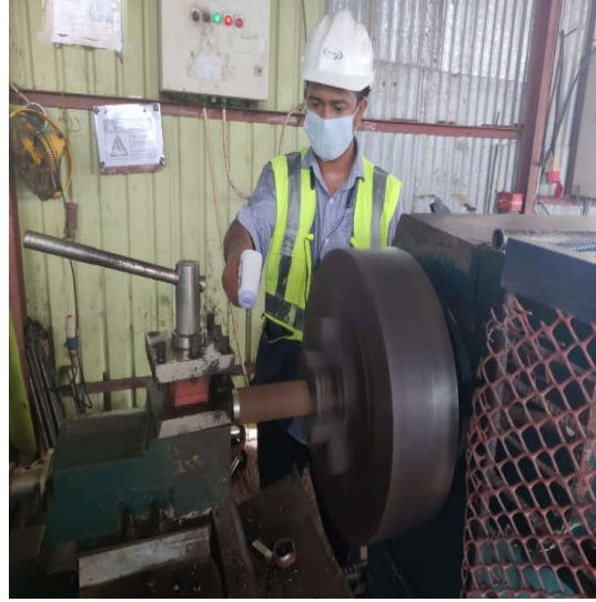
Measuring temperature Using laser type temperature gun.
