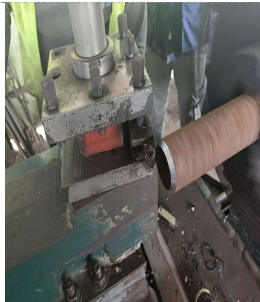
Preparing bevel using Neutral Rake angle Right hand cutting tool
