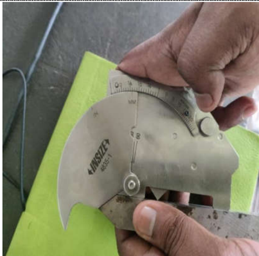
Measuring side flank angle using Multi-functional Weld gauge.
