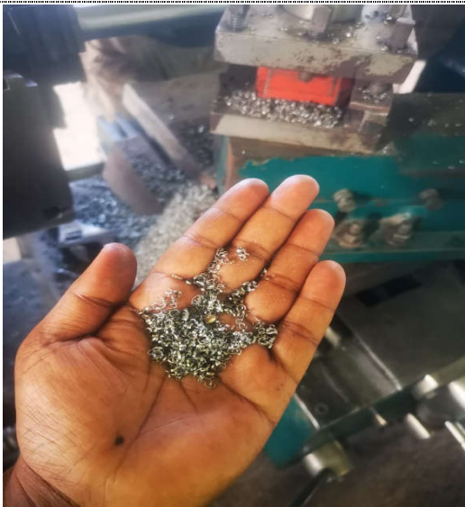
Discontinuous chips found using negative rake angle as well as high power cut.
