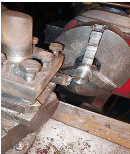
Turning operation for 42 mm dia Reinforcement to prepare Pinion
