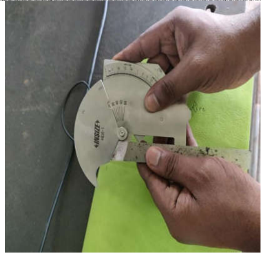
Measuring End cutting edge angle using weld gauge.
