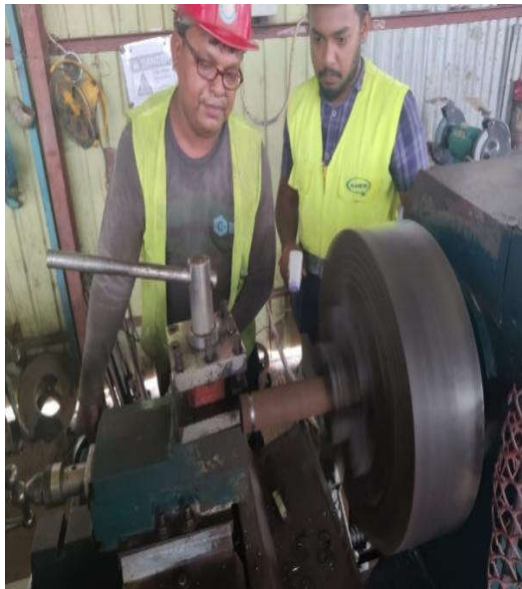
Observing Turning operation, Cut off as well as preparing bevel single bevel.
