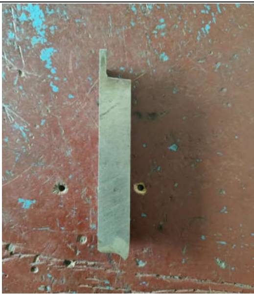
Cut off or parting tool, used for thread cutting, Neutral rake angle
