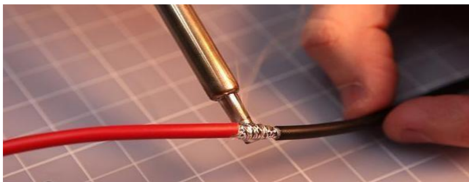
Fig 3.18 Soldering two wires
