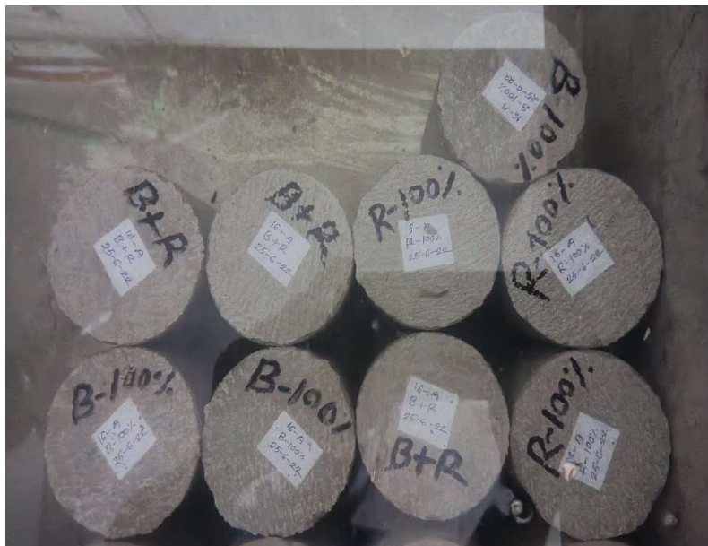
Figure 3.6: Curing of concrete specimens
