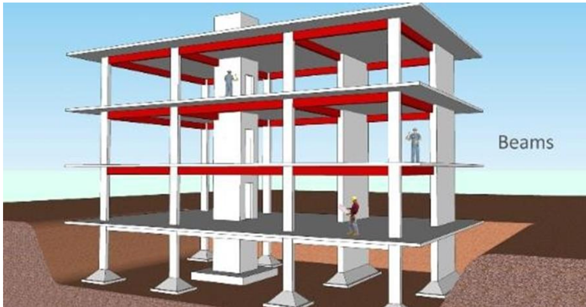
Fig 2.1: Beam Sections in a frame Structure
