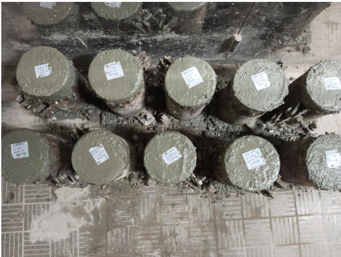
Figure 4.3 Casting in Lightweight Concretes of Cylinder
