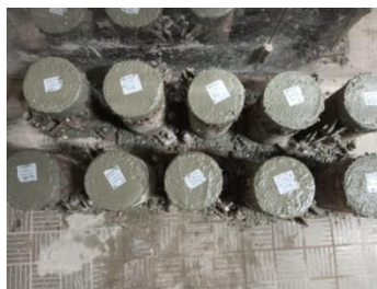
Fig 1.1 : Casting In Cylinder With EPS BEADS
