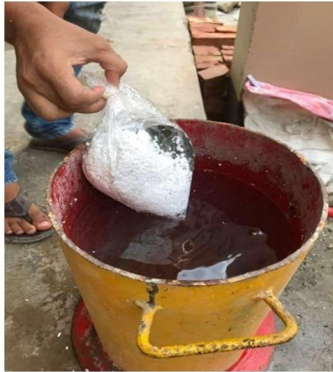
Figure 3.2 Density measurement of EPS beads
