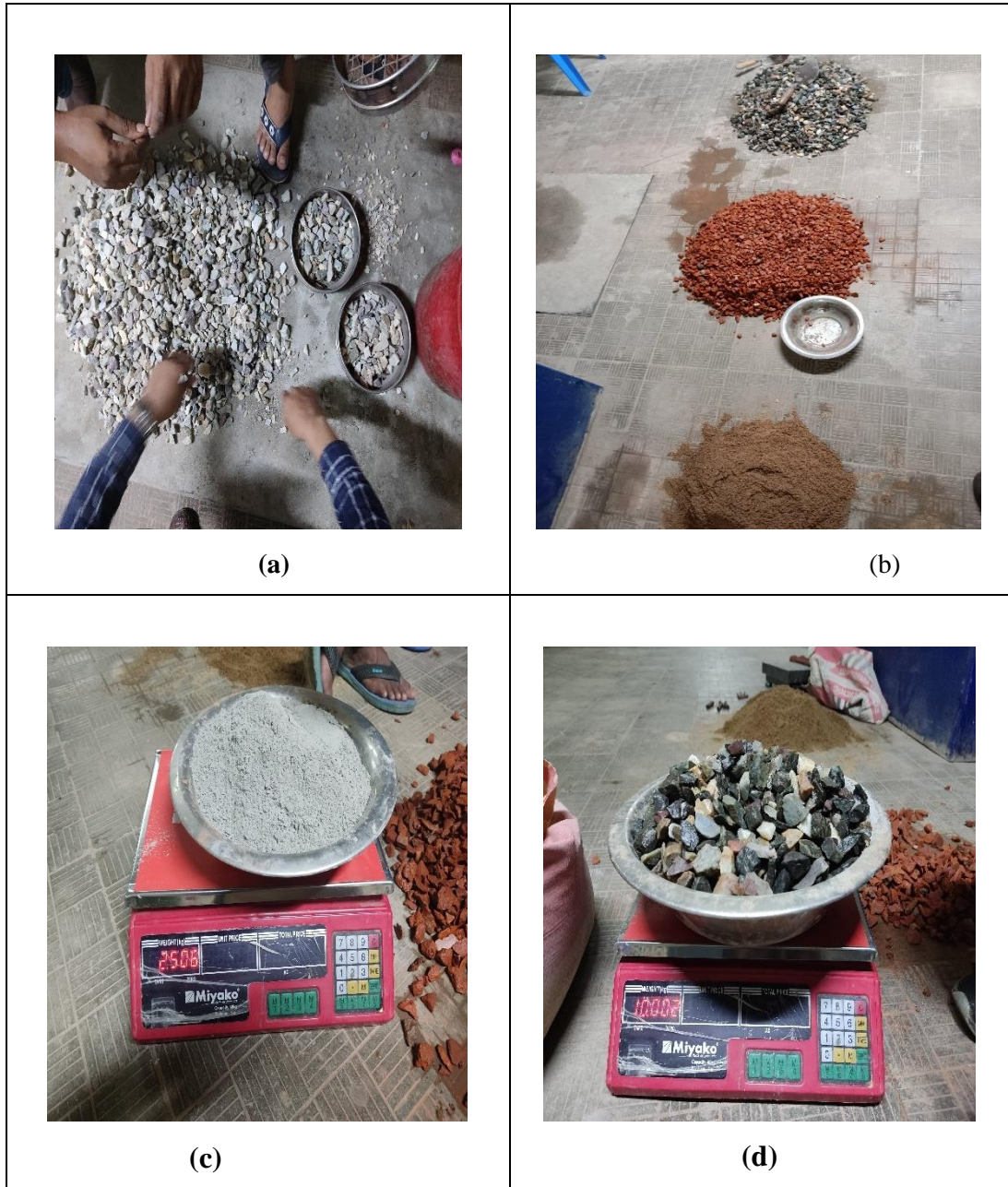
Figure A- 1: a) Stone Broken & Sieved. b) Stone, Bricks, Sand curing after. c) Cement weight measurement for concrete . d) SSD Stone weight measurement for concrete.
