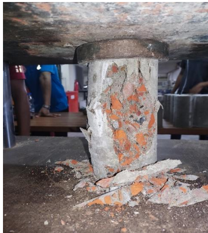
(a) Without Rebar
