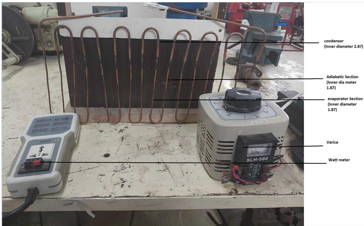
Figure 3 Dual diameter pipe view
