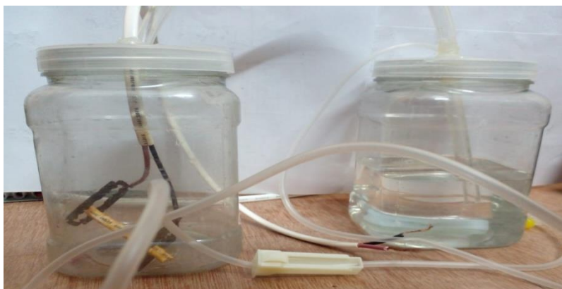
Figure 3.4: Reservoir Tank and PEM Electrolyzer
