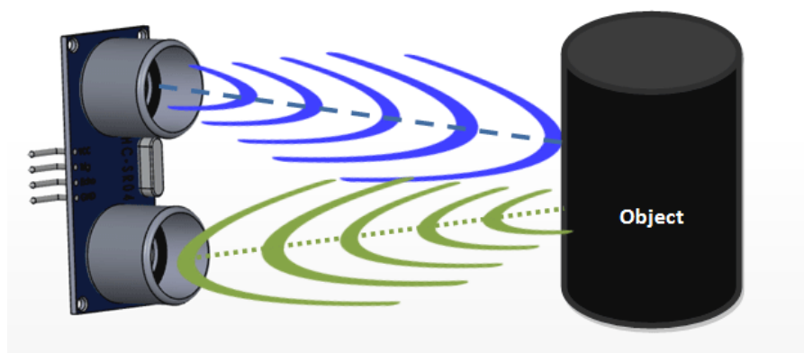
Figure 3.19: Ultrasonic Sensor Working Procedure
