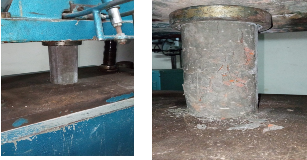
Figure 3.7: Compressive Strength Test
