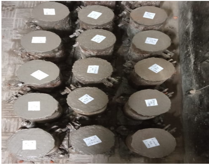
Figure 3.4: Mold of Cylinder.
