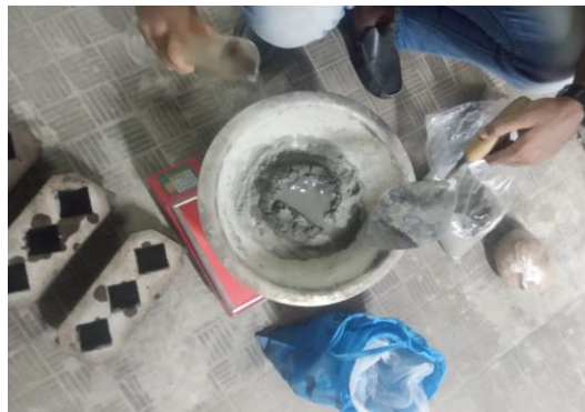
Figure 3.3: Cement mortar Block Molding
