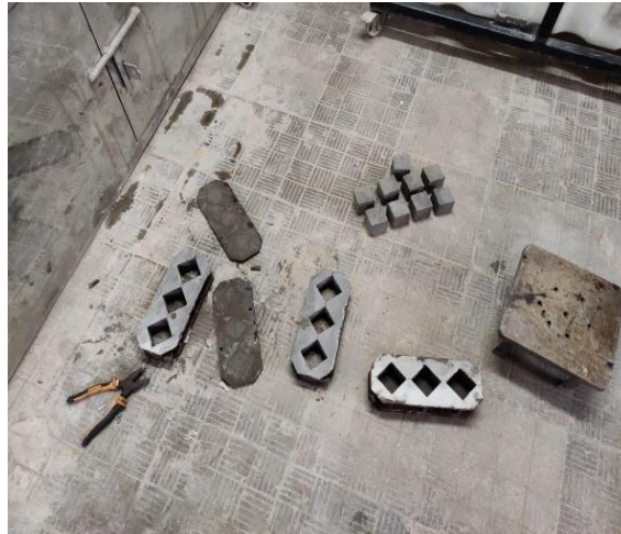
Figure 3.4: Remolding Cement Block
