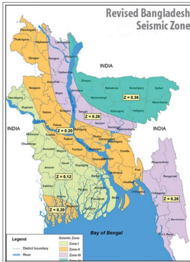
Figure 3: Seismic Zone Coefficients (Ref.: BNBC 2020 Page No: 3117)
