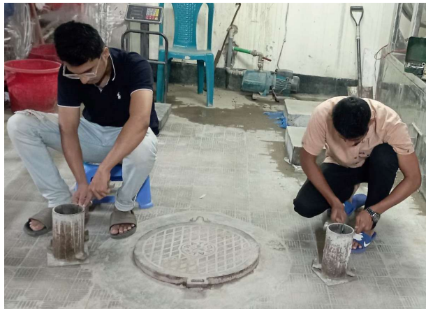
Figure 3.4: Preparing Cylinder Formwork.
