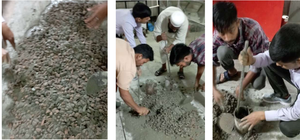
Figure 3.7: Casting of Cylinder.
