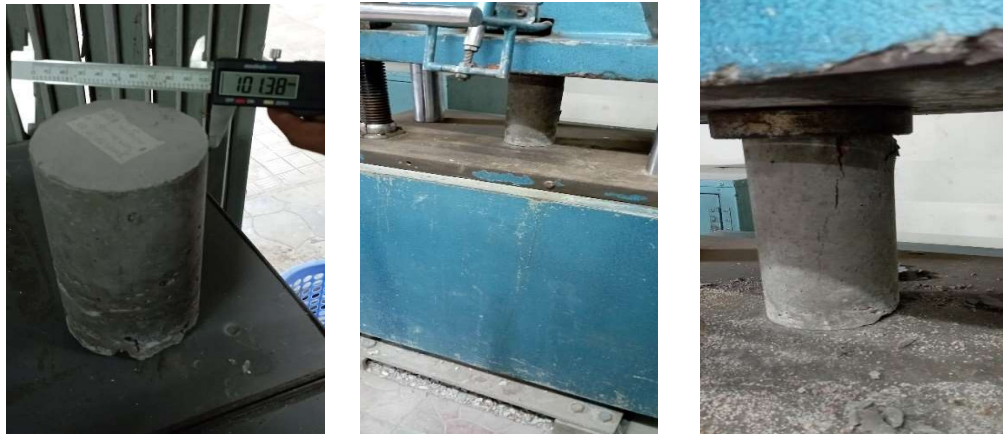
Figure 3.9: Preparation of Cylinder to Crush.
