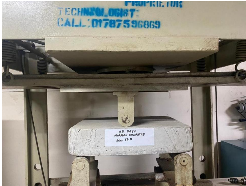
Figure 3.12 : Flexural Strength Test Set-up (Normal Concrete Slab 28 Days)
