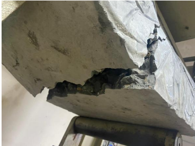
Figure 3.22 : Bending Test Results on Steel Wire Meshes Reinforced Concrete (28 Days)
