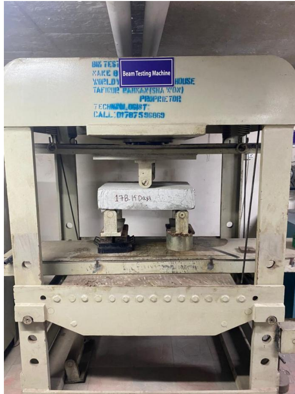
Figure 3.10 : Flexural Strength Test Set-up (Normal Concrete Slab 14 Days)
