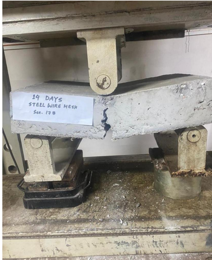
Figure 3.18 : Bending Test Results on Steel Wire Meshes Reinforced Concrete (14 Days)
