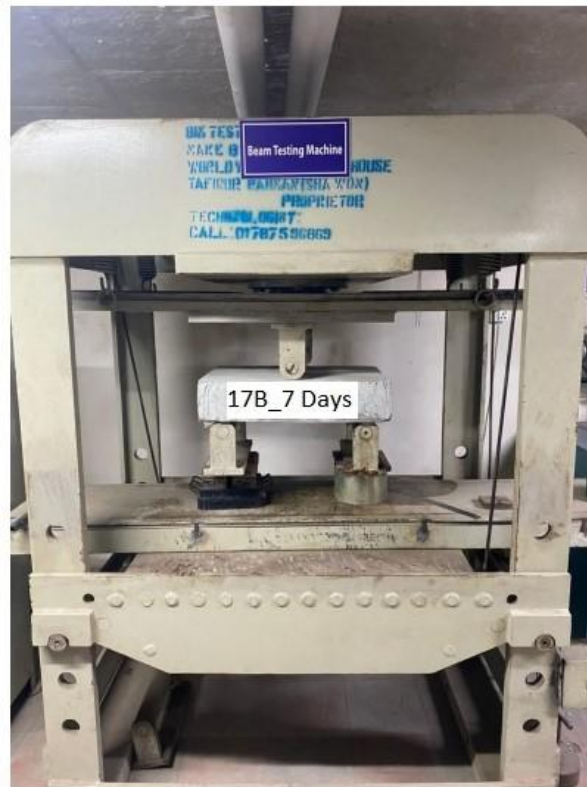
Figure 3.8 : Flexural Strength Test Set-up (Normal Concrete Slab 7 Days)
