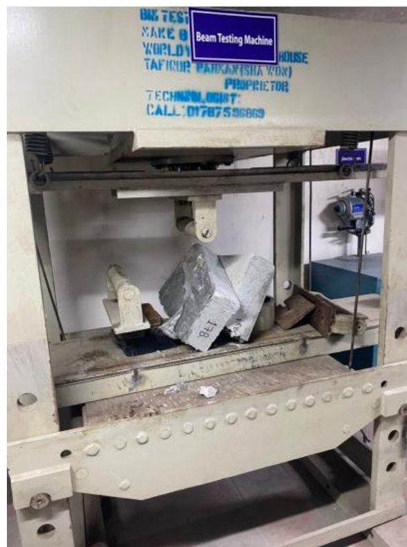
Figure 3.9 : Test Results on Normal Concrete Slab (7 Days)
