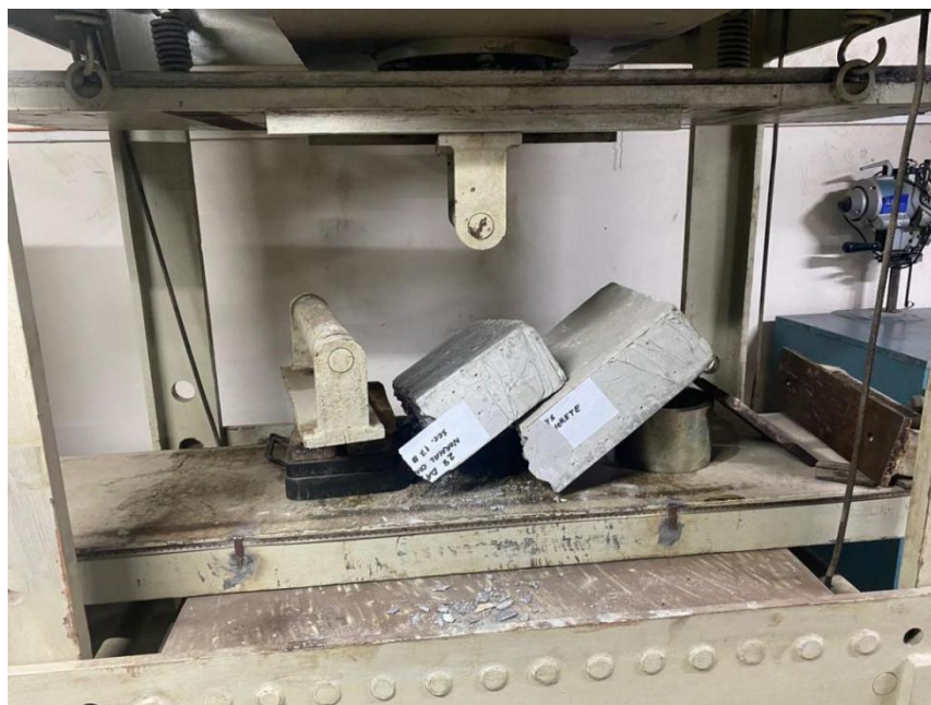
Figure 3.13 : Test Results on Normal Concrete Slab (28 Days)
