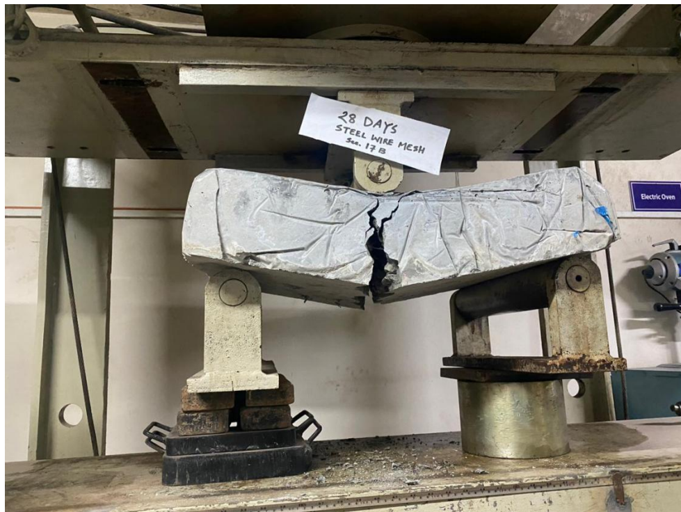
Figure 3.21 : Bending Test Results on Steel Wire Meshes Reinforced Concrete (28 Days)
