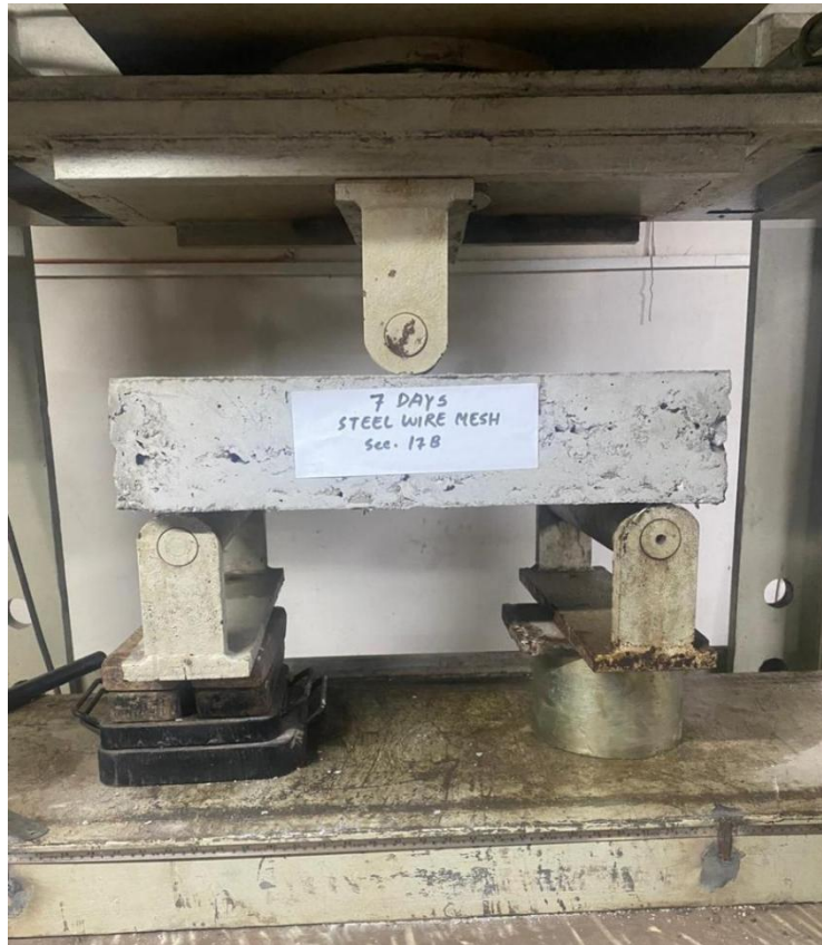
Figure 3.14 : Flexural Strength Test Set-up (Steel Wire Mesh Concrete Slab 7 Days)
