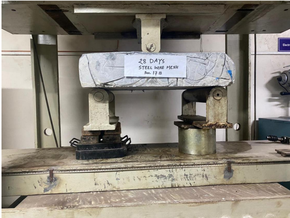
Figure 3.20 : Flexural Strength Test Set-up (Steel Wire Mesh Concrete Slab 28 Days)
