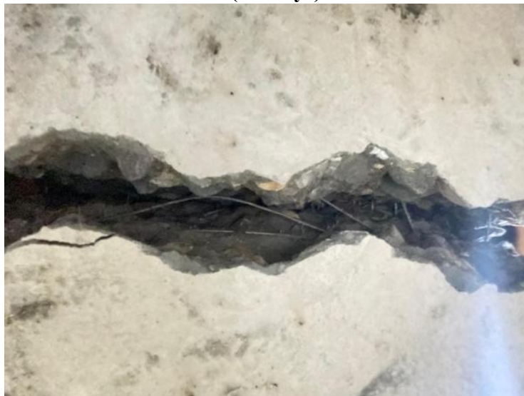
Figure 3.23 : Bending Test Results on Steel Wire Meshes Reinforced Concrete (28 Days)
