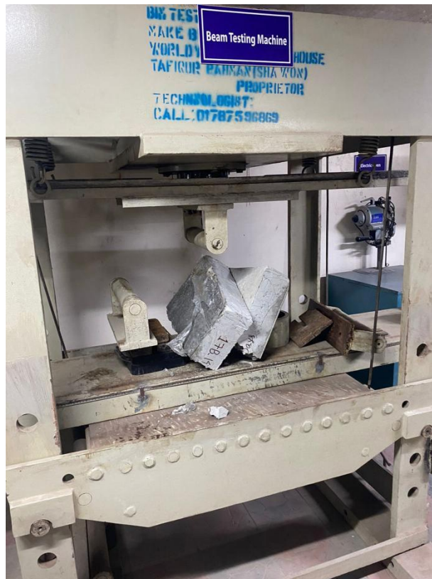
Figure 3.11 : Test Results on Normal Concrete Slab (14 Days)
