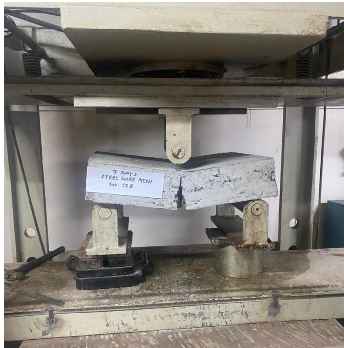
Figure 3.15 : Brnding Test Results on Steel Wire Meshes Reinforced Concrete (7 Days)
