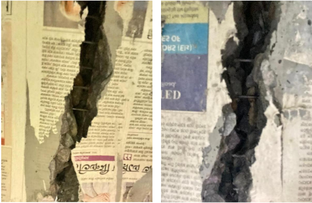
Figure 3.16 : Bending Test Results on Steel Wire Meshes Reinforced Concrete (7 Days)
