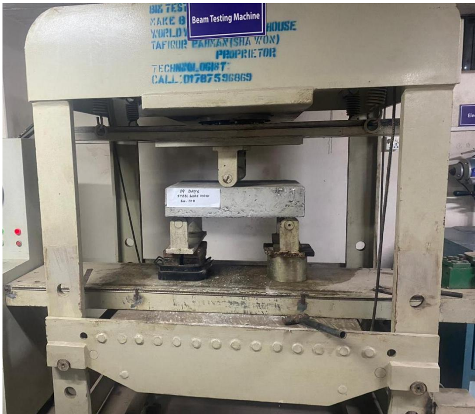
Figure 3.17 : Flexural Strength Test Set-up (Steel Wire Mesh Concrete Slab 14 Days)
