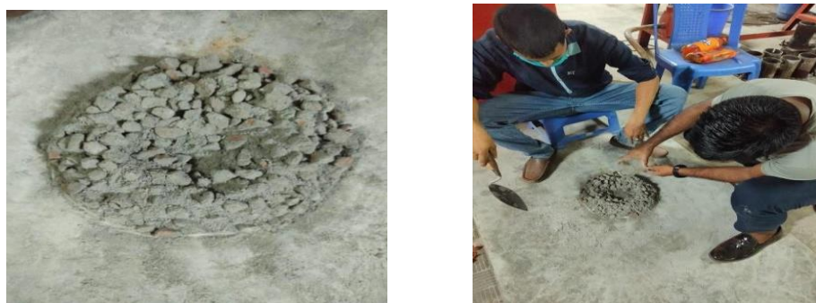
Figure 3.9: Mixing of aggregate.
