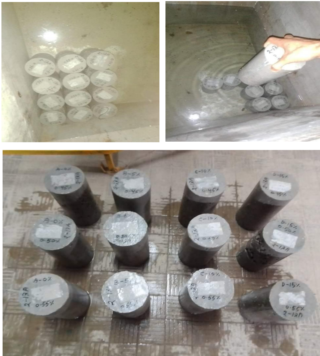
Figure 3.15: Curing The Cylinder.
