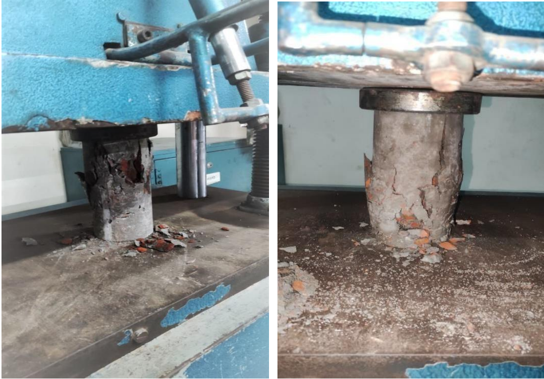
Figure 4.1: Different types of failure mode of the concrete cylinder.
