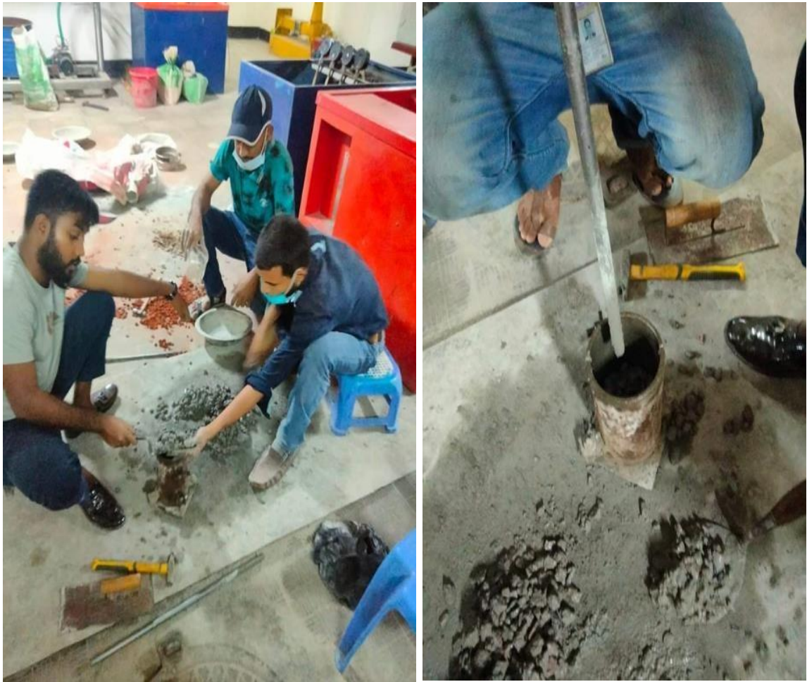
Figure 3.13: Concrete placing & Compaction.
