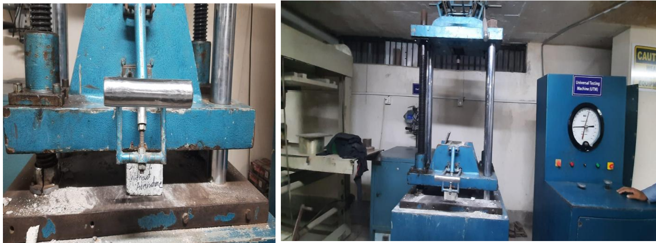
Figure 3.6: Typical setup for compressive strength determination
