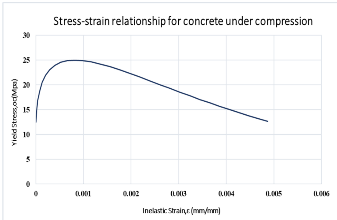
Figure 3:6 Stress-strain relationship for concrete under uniaxial compression
