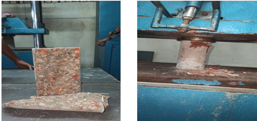
Figure 3.11 After Crushed Cylinder
