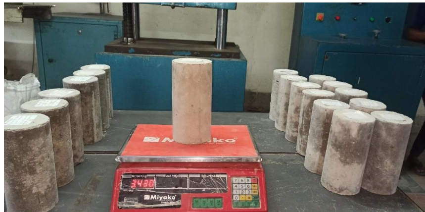
Figure 3.9 Preparation to Crush of Cylinder
