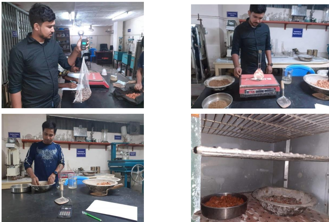
Figure 3.4 Specific Gravity and Absorption Capacity of Coarse Aggregate
