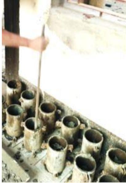
Figure 3.9: Tamping of cylindrical mold
