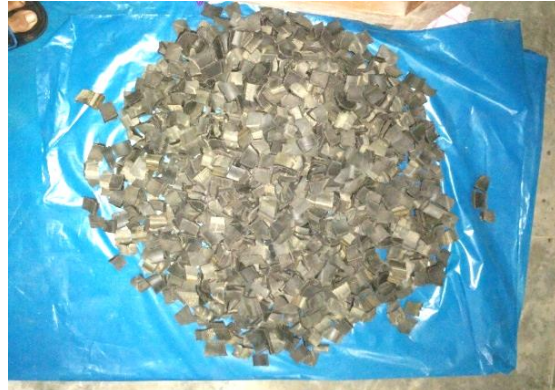
Figure 3.2: After cutting waste tyre
