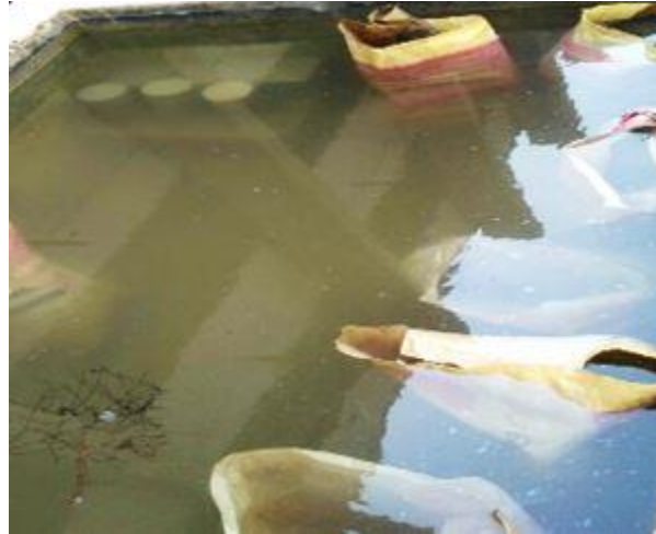
Figure 3.12: Curing the specimen
