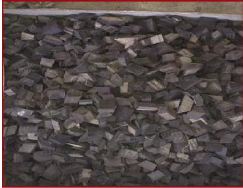
Figure 2.3: Waste tyre as coarse aggregate (Engineering Science and Technology, an International Journal; February 2017)
