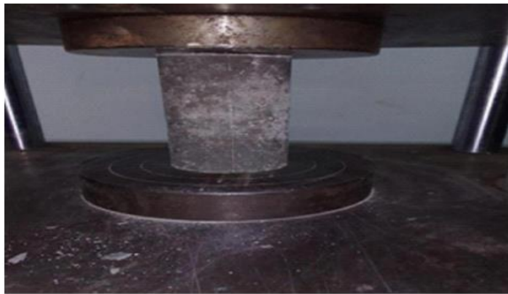
Figure 3.9: Set up for Compressive Test
