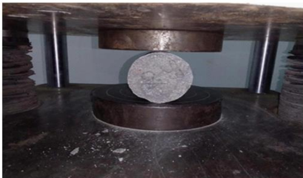
Fig 3.11: Set up for Tensile Strength
