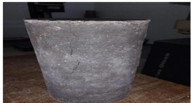
Figure 3.10: Compressive Failure Pattern
