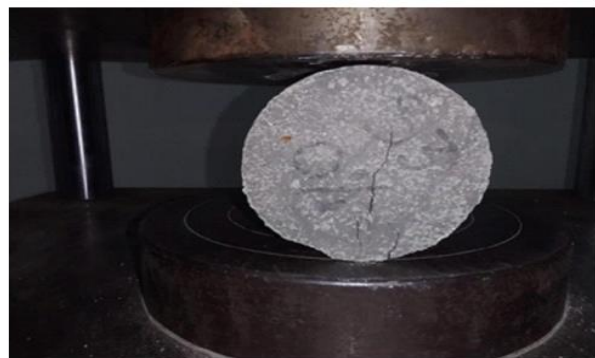
Fig 3.12: Failure pattern for Tensile Strength
