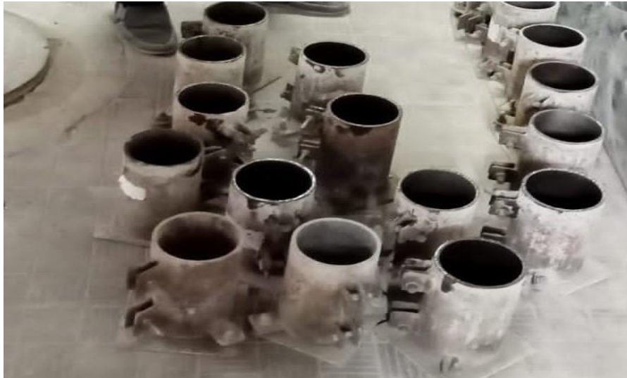
Fig. 3.1(b): Mold Ready for Casting
