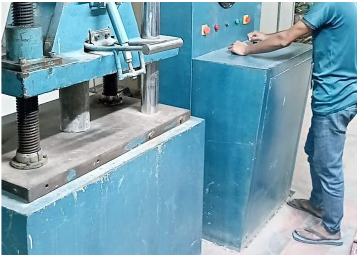
Fig. 3.6: Place the cylinder in UTM machine.
