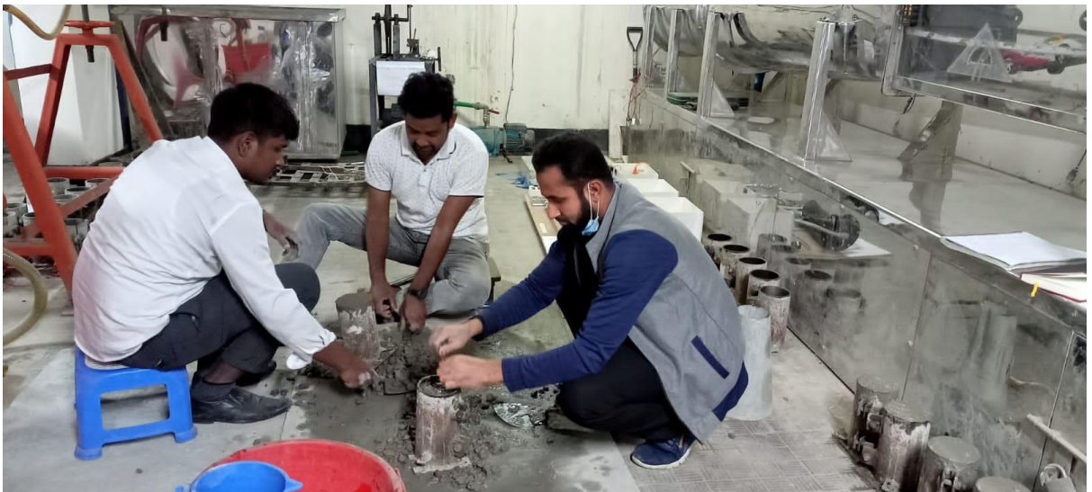
Fig. 3.3: Casting of Cylinder
