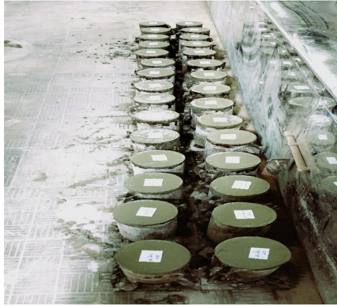
Figure 3-10 Cylinder After Casting.
