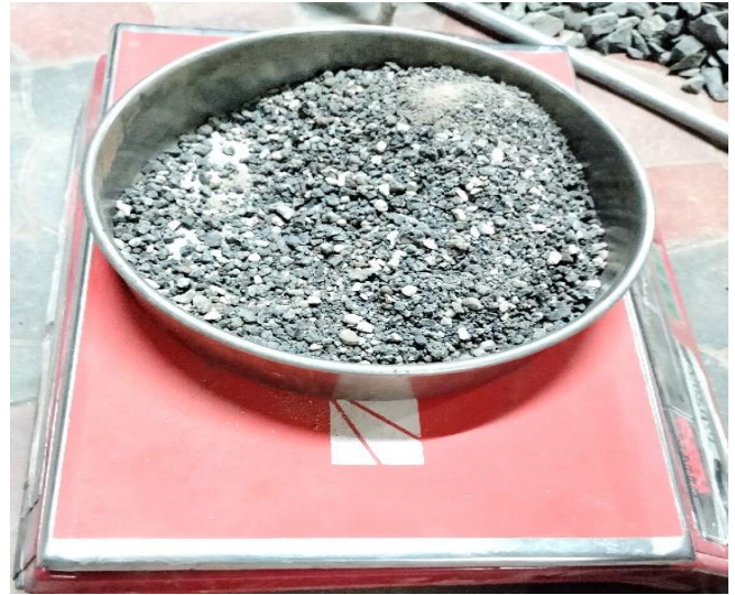
Figure 3-4 Partially Replaced Recycled Fine Aggregate (Slag)
