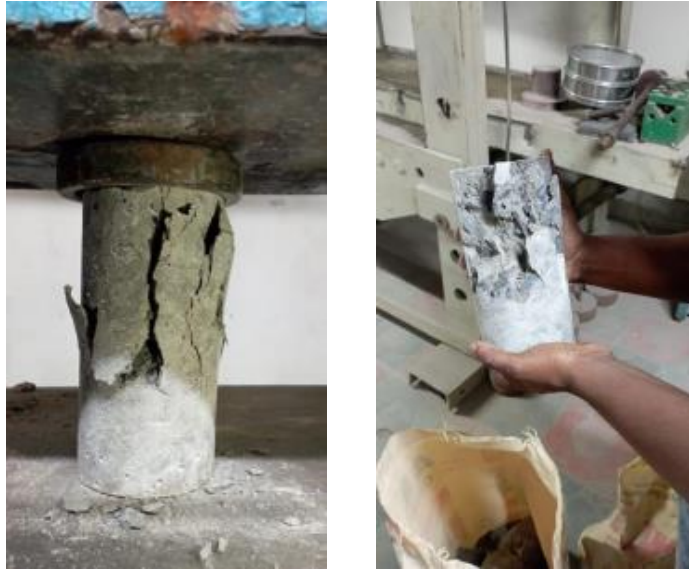
Figure-7: Concrete Cylinder after Crushing
