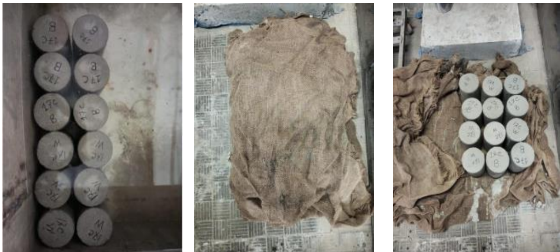
Figure-6: Immersion and Wet Covering Curing Method of Concrete Cylinders
