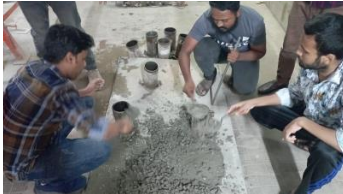
Figure-4: Preparing of Molds- Cleaning works
