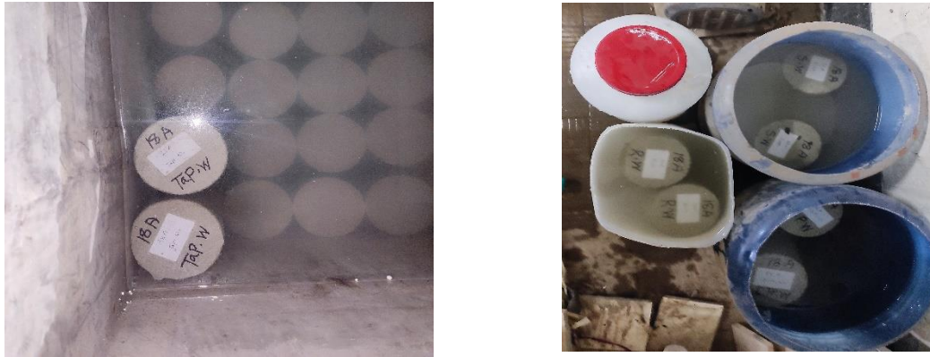
Figure 9: Curing of concrete specimens in various water (Lab)
