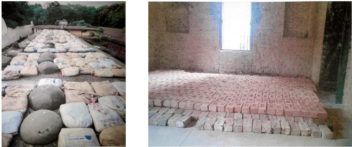
Fig 4.8: Slab Strength Analysis: Brick Laying/Sand Bag Test
