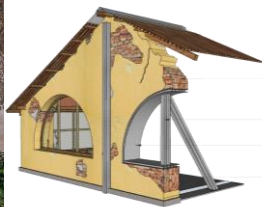
Strengthening the broken part with metal bracing
