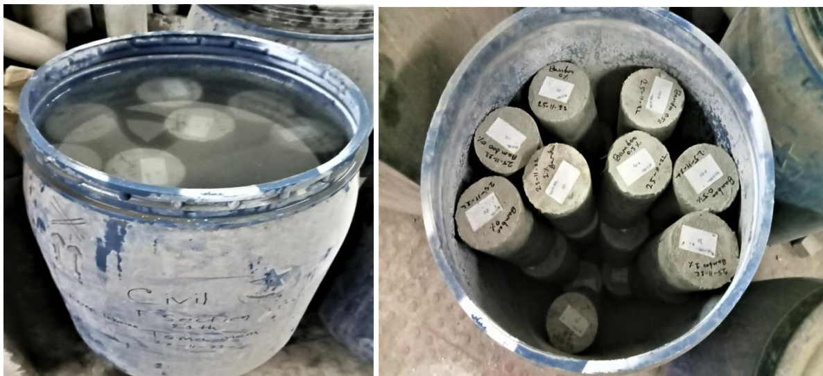
Figure 3.6: Curing of Concrete
