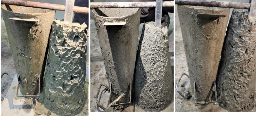
Figure 2.10: Slump test for 0%, 0.5% & 1% Ratio of Bamboo fiber mixed Concrete.
