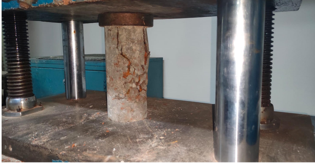
Figure: 1.17 Compressive Strength Testing
