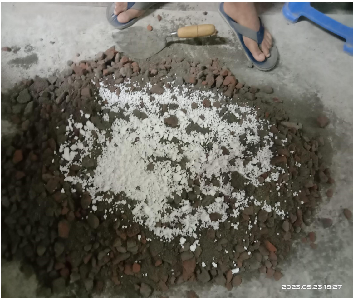
Figure: 1.9 Concrete mixed with Expanded Polystyrene Beads (EPS)
