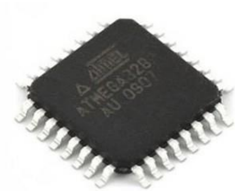
Figure 3.4: Micro controller IC AT mega 328p
