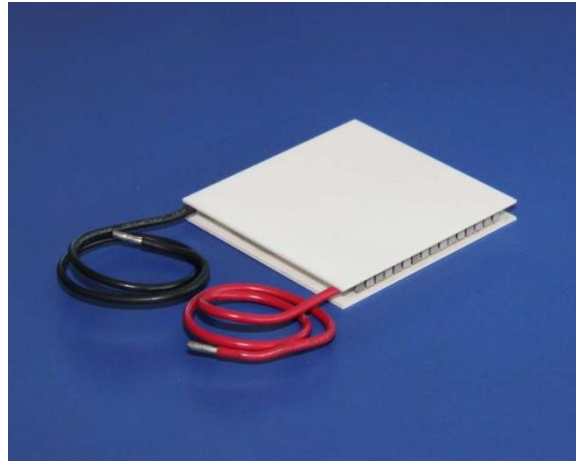
Fig 3.5: Picture of Peltier Module. [22]
