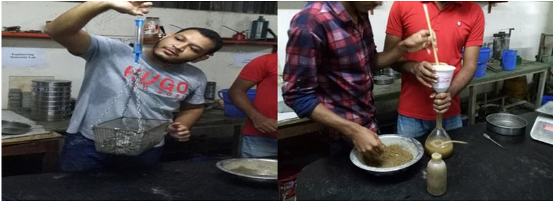
Figure 3.2: Determination of Specific Gravity
