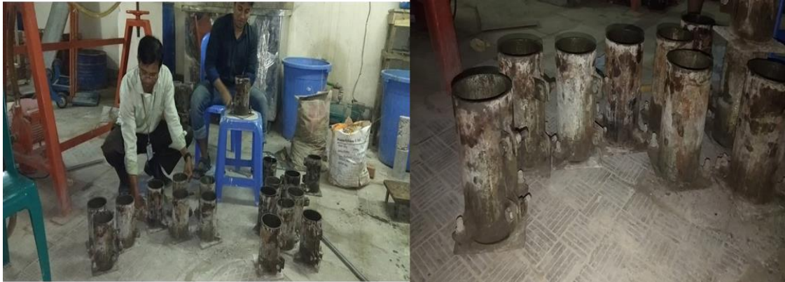
Figure 3.4: Preparation of Cylinder Mold
