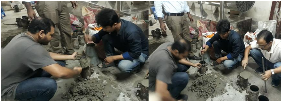
Figure 3.6: Filling the Cylinder Mold by Weight Materials
