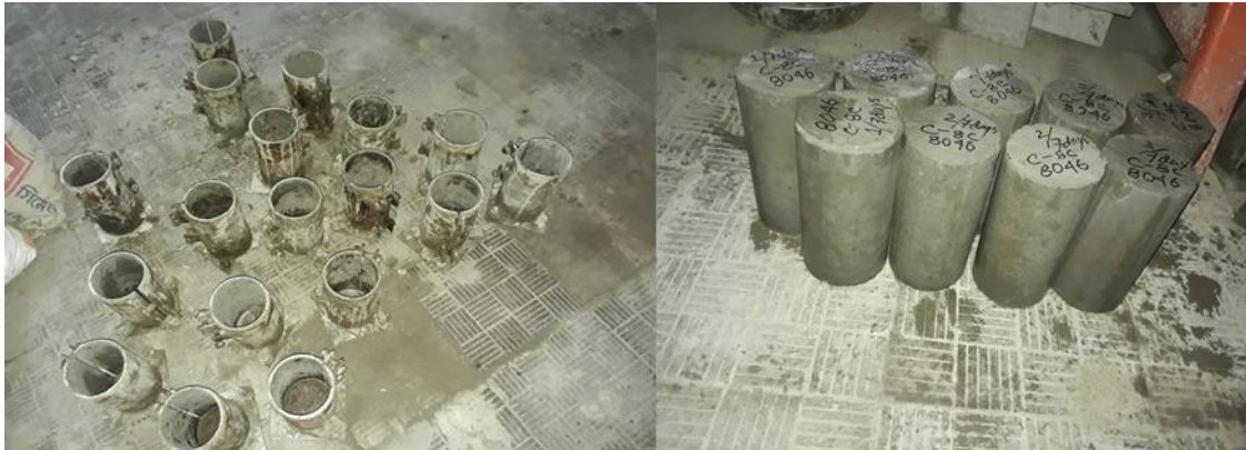
Figure 3.10: De Molding of Cylinder
