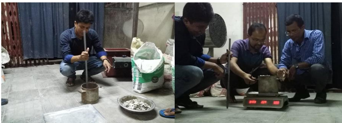
Figure 3.3: Determination of Unit Weight of Coarse Aggregate
