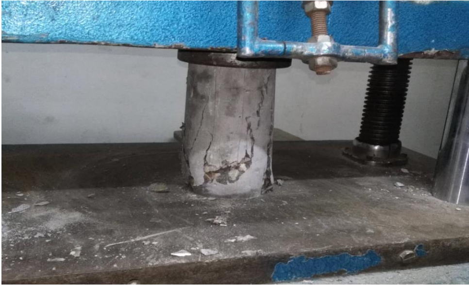
Figure 5.4: Failure Pattern Columnar of Angular Shape Stone Chips on Compression
