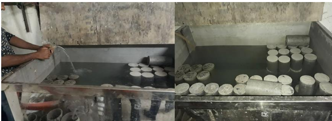
Figure 3.11: Curing of Cylinder
