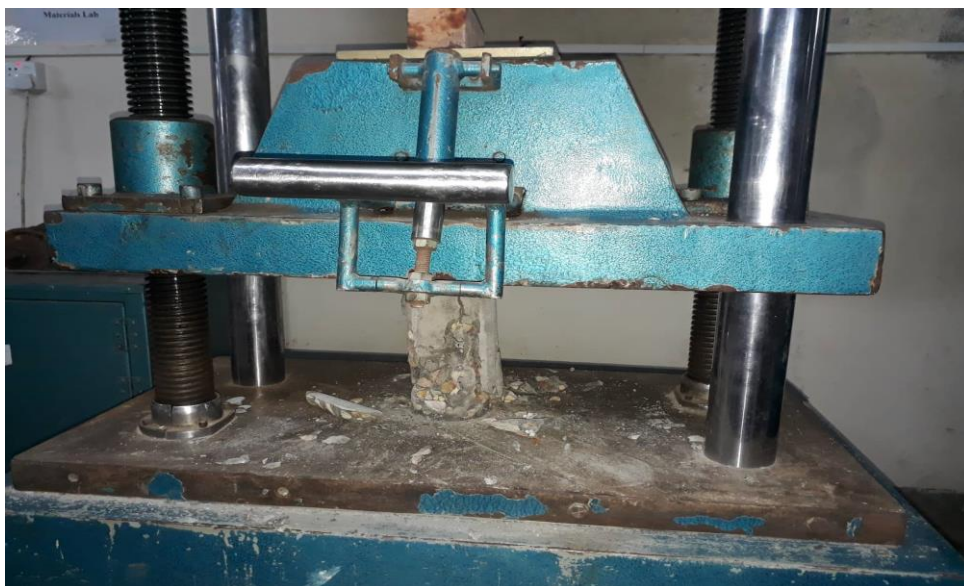
Figure 5.3: Failure Pattern Shear of Round Headed Stone Chips on Compression
