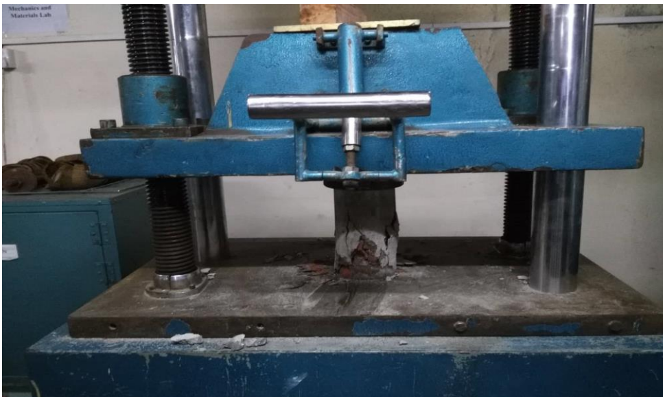
Figure 5.5: Failure Pattern Cone and Shear of Brick Chips on Compression
