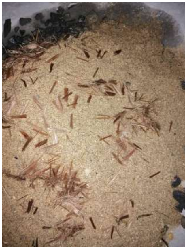
Figure 8: Concrete Mixing With Jute Fibre
