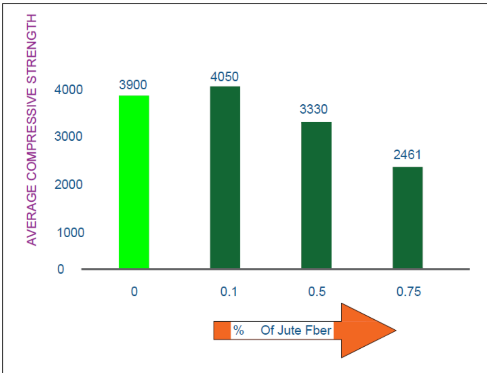
Figure :26 After 28 days compressive strength =4000 psi (Jute Fiver Length=15mm)
