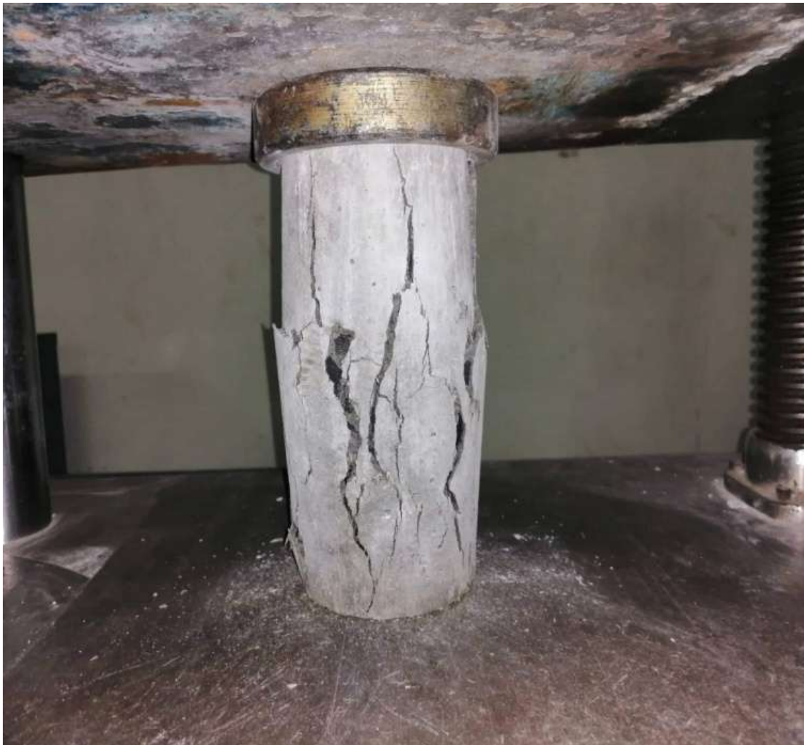
Figure 1: Compressive Strength Test
