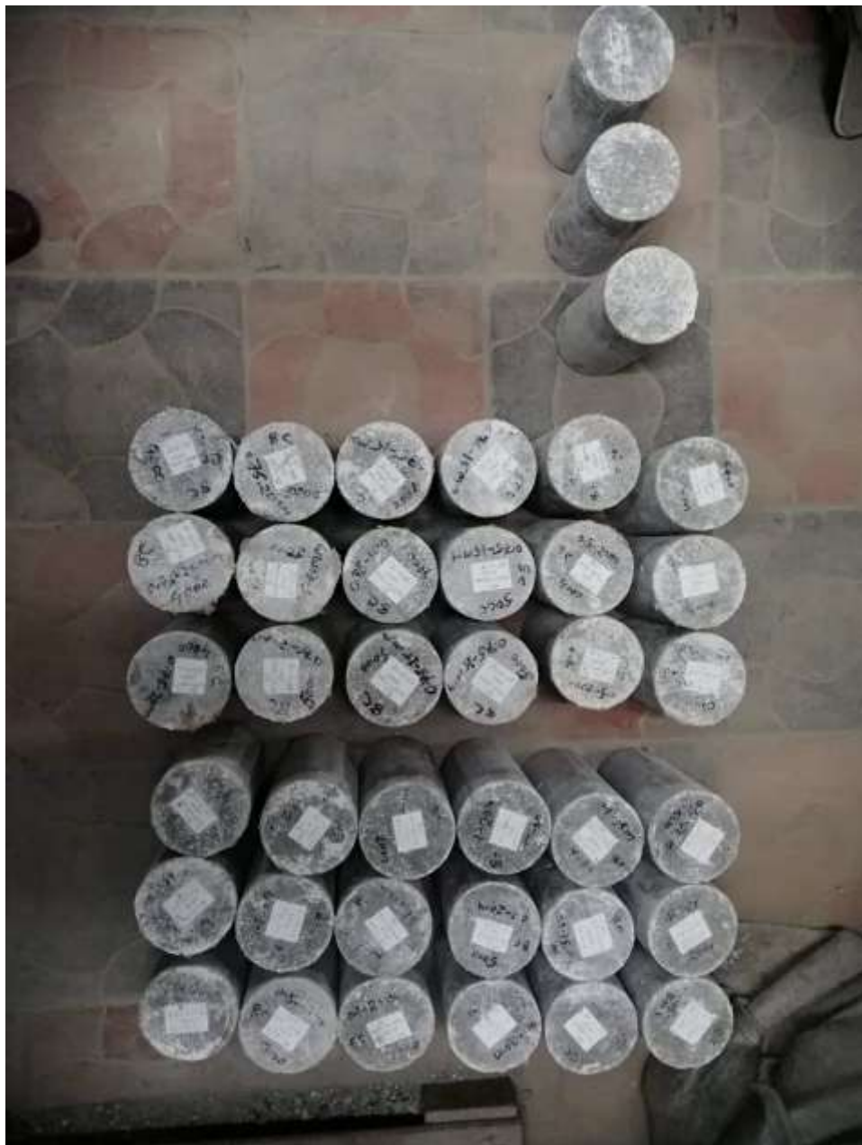
Figure 14: After 28 days with draw from the water dram of cylinder
