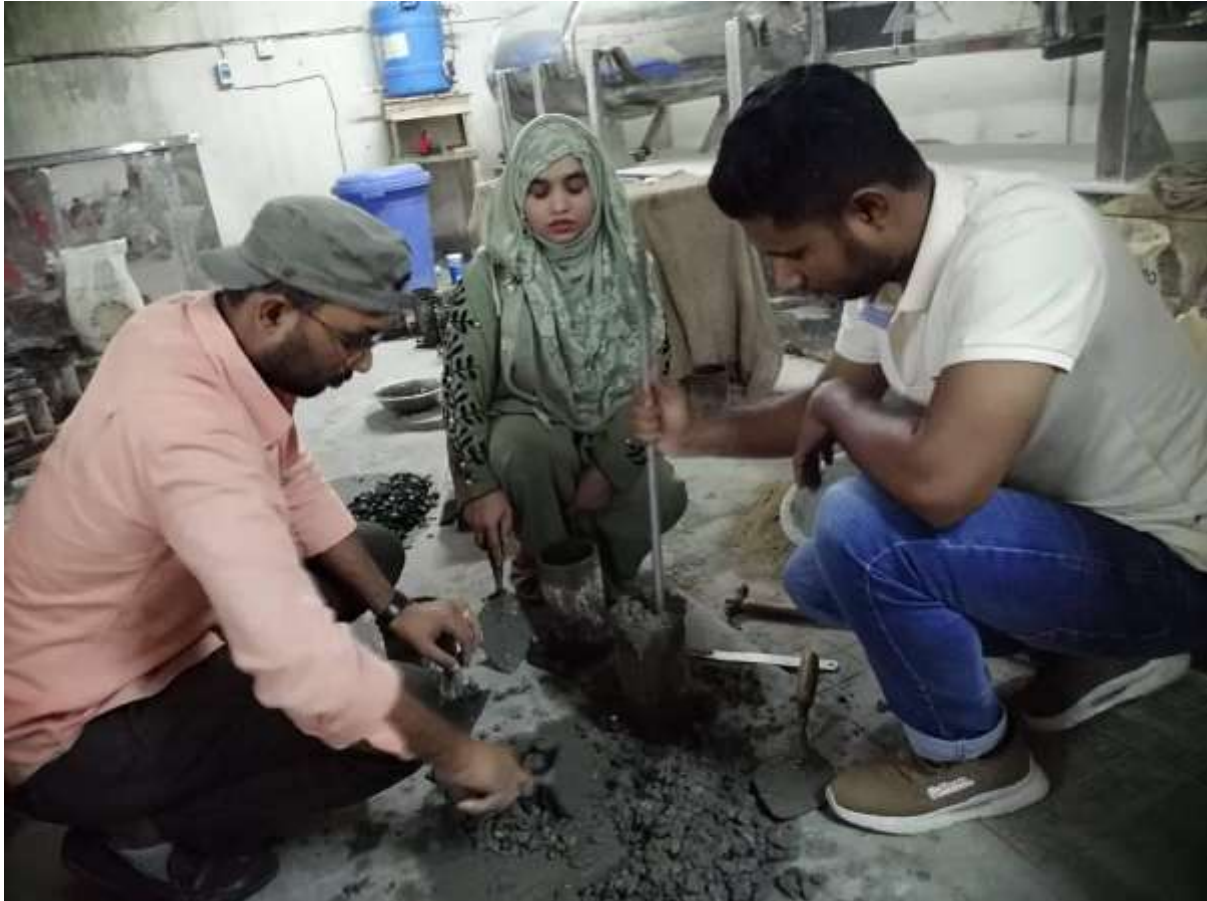
Figure 16: Tamping Of Cylinder Specimen
