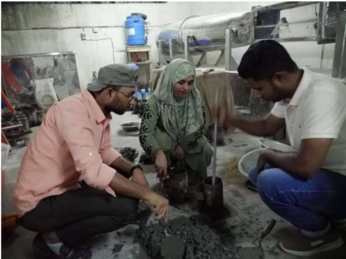
Figure 13: Preparation of concrete cylinder
