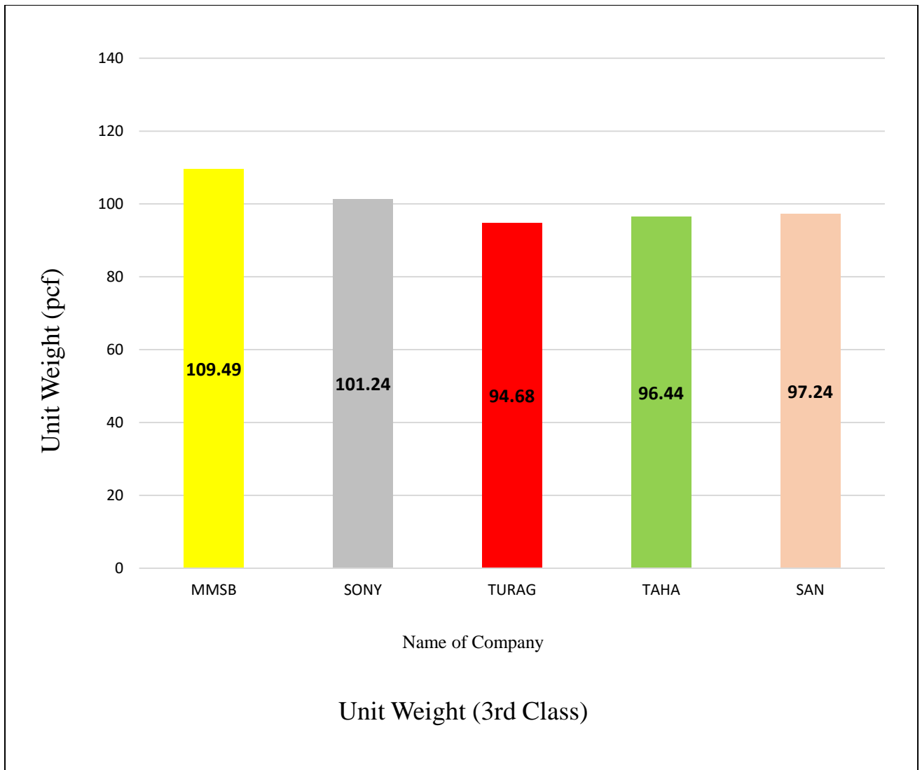
Fig -4.16: "Unit weight test calculation" For 3rd Class Brick
