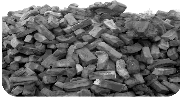
Fig -2.12 Over Burnt or Jhama Brick
