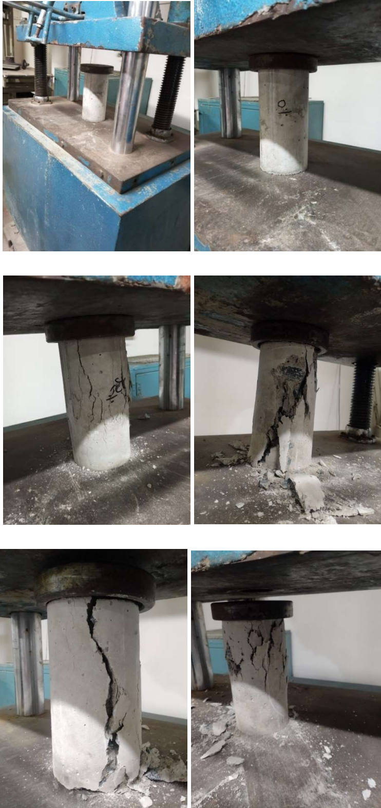
Fig 3.11: Pictures of specimen testing of compressive strength using UTM
