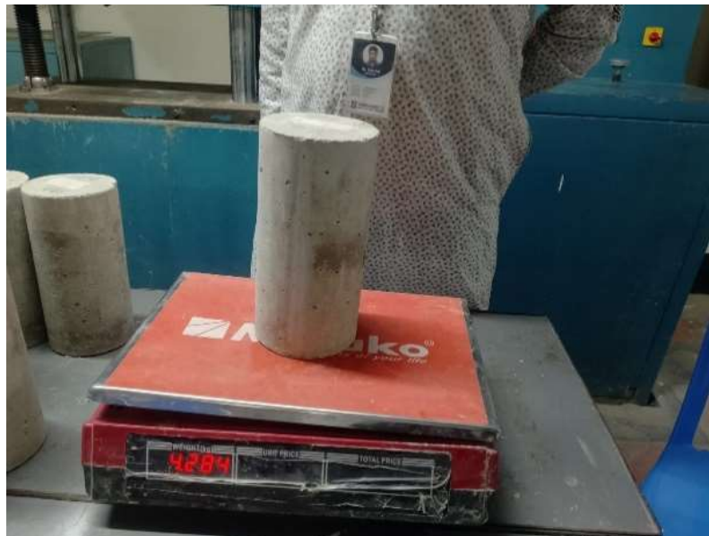
Fig 3.10: Measuring the weight of specimen for unit weight calculation
