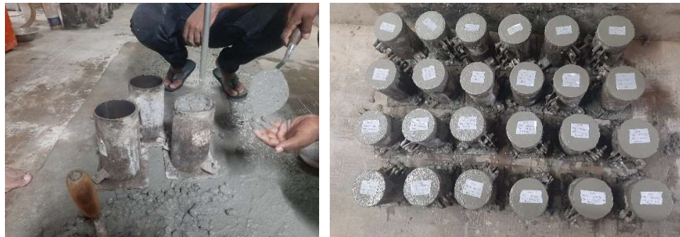
Fig 3.7: Concrete specimen casting in Cylinder
