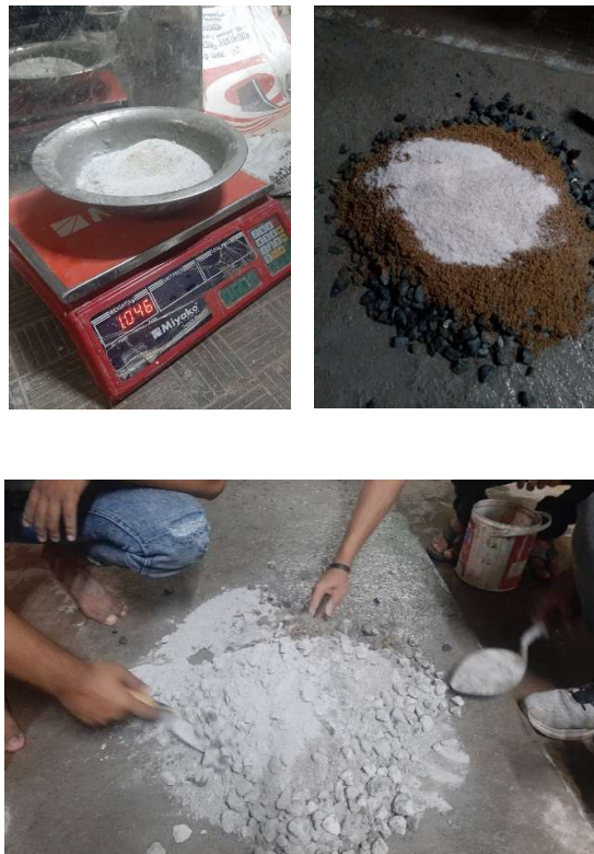
Fig 3.6: Concrete With Waste Glass As Partial Sand Replacement Mixing.
