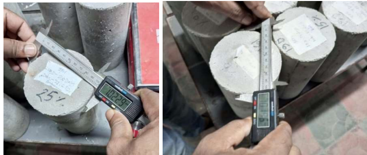
Fig 3.9: Measuring specimen before testing for compressive strength
