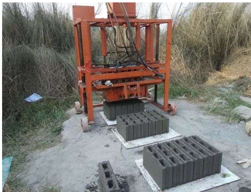
Figure: 1.2 Hollow Block Concrete Brick Hydraulic Machine
