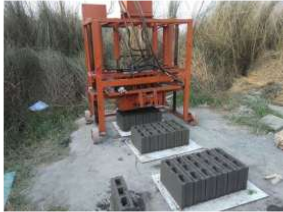
Figure: 1.2 Hollow Block Concrete Brick Hydraulic Machine
