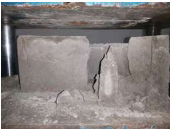
Figure: 1.11 Compressive Strength Test
