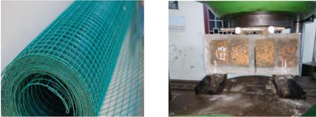
Figure 2.7: G.I (15mm spaced) and Epoxy coated (12mm spaced) locally available mesh & Experimental set up of masonry prism with embedded mesh.
