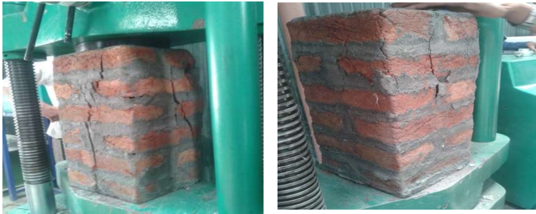
Figure 2. 12: Failure pattern of sample.
