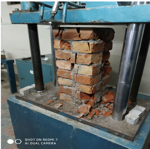
Figure 3. 027: Load arrangement of brick column in UTM.
