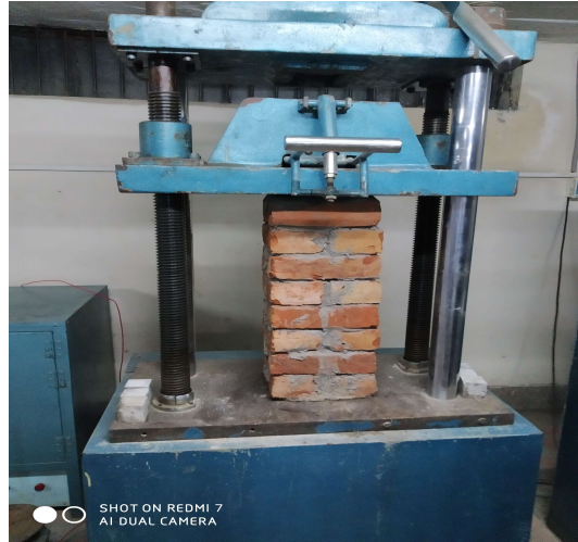
Figure 3. 027: Load arrangement of brick column in UTM.
