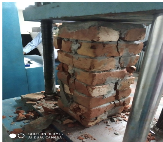
Figure 3. 028: Failure of brick column under UTM machine.
