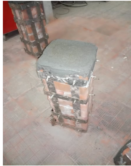
Figure 3. 32: Brick column with steel strip.
