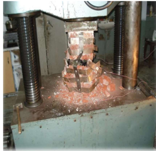
Figure 2. 2: Failure of column strip Under UTM machine.
