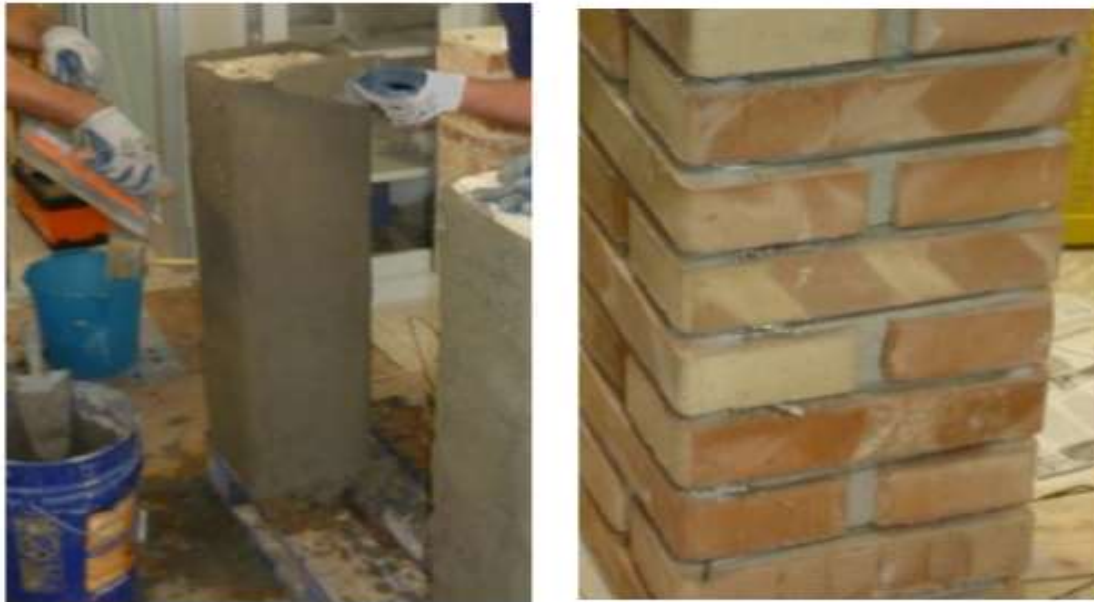
Figure 2. 22: Preparation of specimens: (a) basalt-reinforced specimen; (b) specimen reinforced with steel wires.
