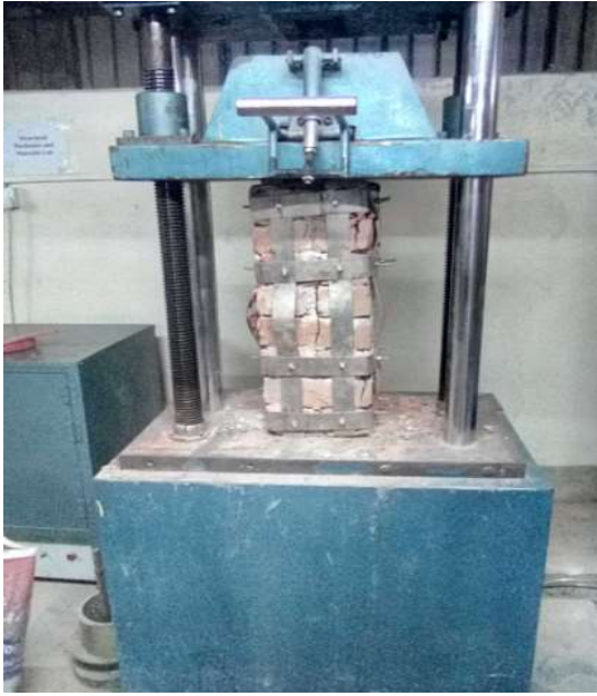
Figure 3. 33: Failure of column strip under UTM machine.
