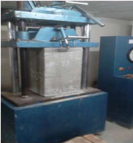
Figure 3. 31: Load arrangement of brick column reinforcement in UTM
