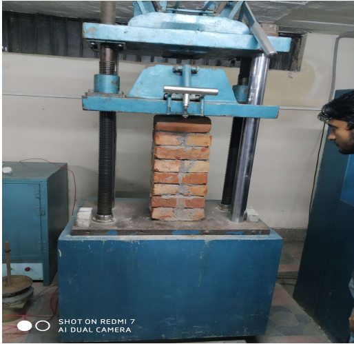
Figure 3. 027: Load arrangement of brick column in UTM.
