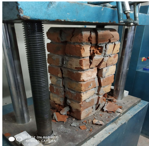
Figure 3. 027: Load arrangement of brick column in UTM.
