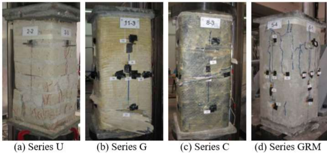
Figure 2. 16: Specimens' failure mode.
