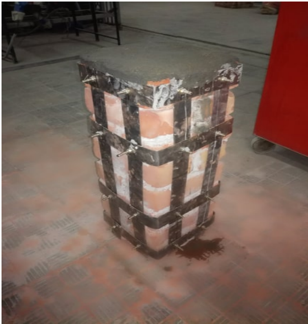
Figure 3. 32: Brick column with steel strip.
