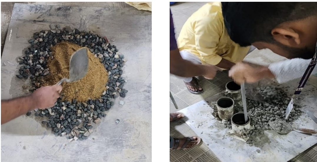
Figure 3-4. Casting of Cylinder.
