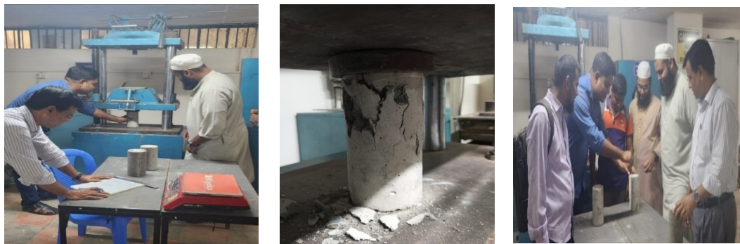
Figure 3-6. Preparation of Cylinder to Crush.
