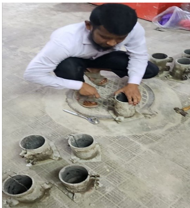
Figure 3-1. Preparing Cylinder Formwork.
