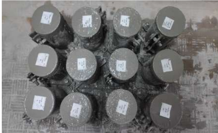
Fig: 3.2.2: Casting Cylinders
