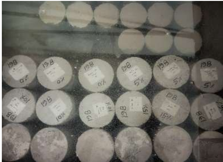
Fig: 3.2.3: Casting Cylinders Curing time
