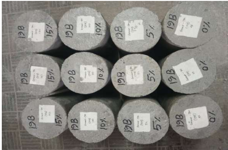
Fig: 3.2.4: Dry Casting cylinders
