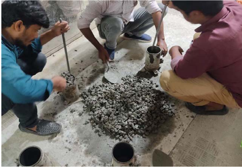
Figure 3-3. Casting of Cylinder
