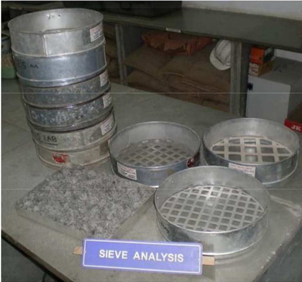
Figure 2-5. Sieve Analysis of Fine and Coarse Aggregate
