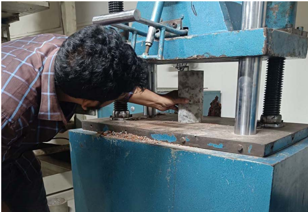
Figure 3-6. Placing the cylinder in UTM machine.
