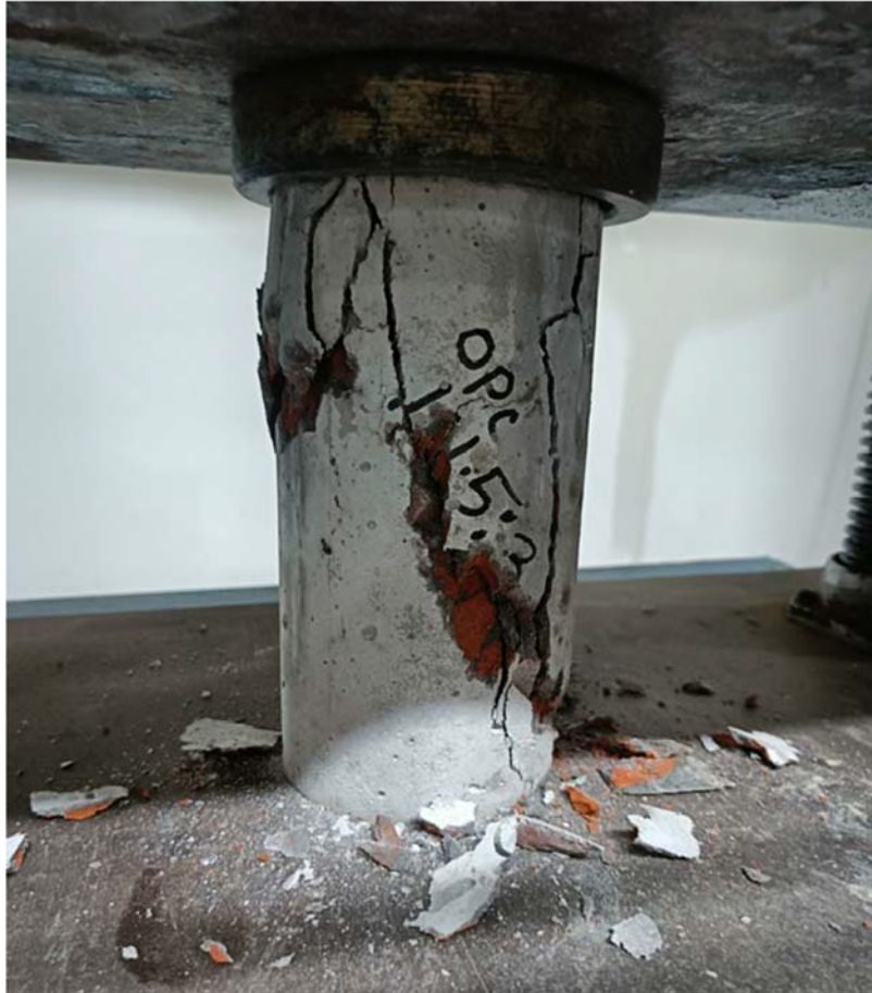
Figure 3-7. Compressive fracture of Cylinder Grade M15 and M20
