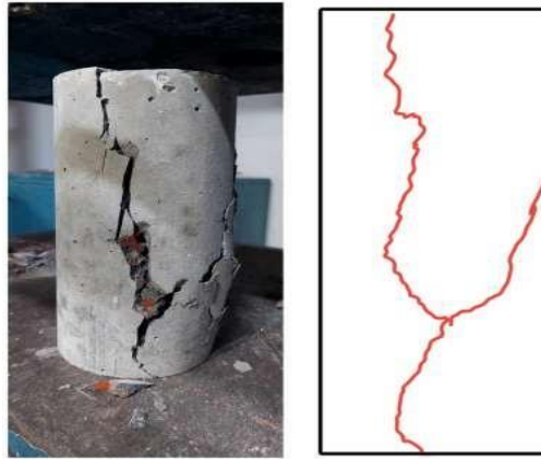
Figure 4.2.1 Failure Type 2 for Concrete type 2. result (90 kn /sqmm)
