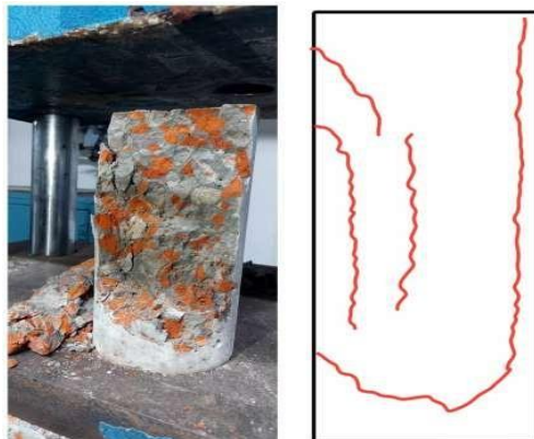
Figure 4.4.2 Failure Type for 2 Concrete type 4. result (109 kn /sqmm)
