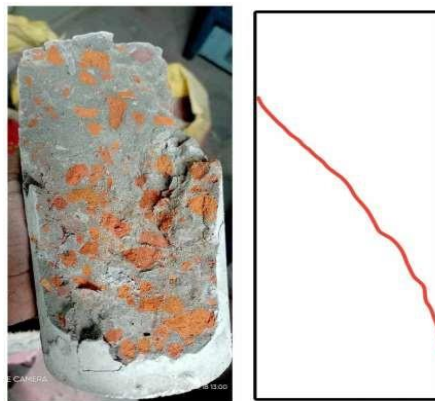
Figure 4.5.2 Failure Type 4 for Concrete type 5 result (105 kn /sqmm)
