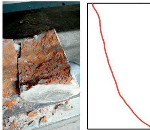
Figure 4.7.2 Failure Type 4 for Concrete type 7 result (118 kn /sq mm)
