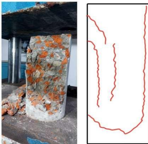
Figure 4.3.3 Failure Type 4 for Concrete type 3. result (99 kn /sqmm)
