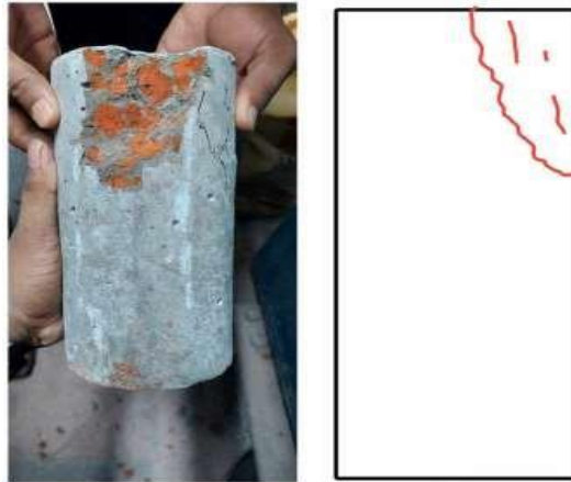
Figure 4.1.1 Failure Type 5 for Concrete type 1. result (83) KN/sq mm
