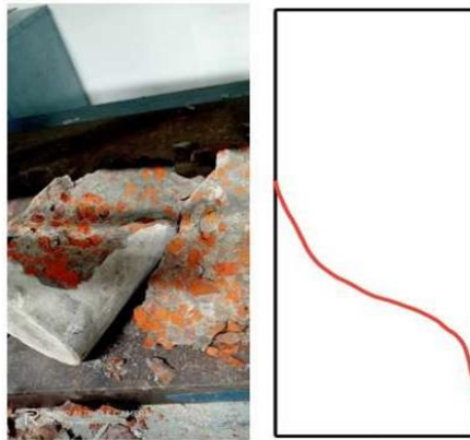
Figure 4.5.1 Failure Type 4 for Concrete type 5 result (118 kn /sqmm)
