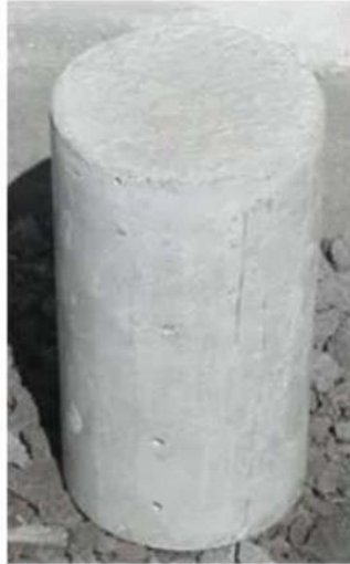
Figure.2.3 Concrete Cylinder for Compression Test
