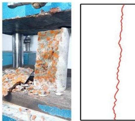
Figure 4.3.2 Failure Type 3 for Concrete type 3. result (109 kn /sq mm)
