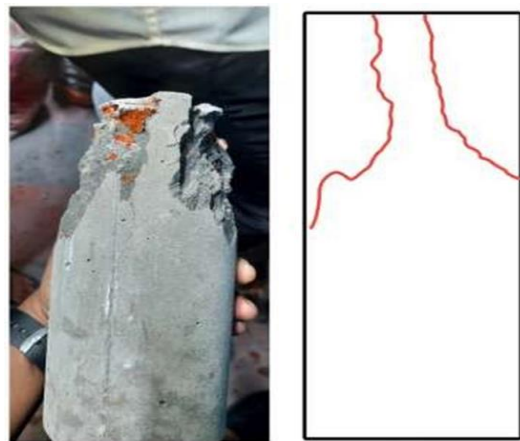
Figure 4.1.2 Failure Type 2 for Concrete type 1. result (92) kn /sqmm
