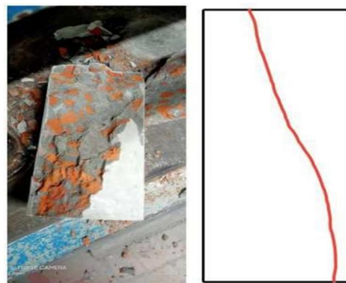
Figure 4.7.3 Failure Type 3 for Concrete type 7. result (140 kn /sqmm)
